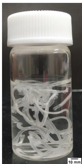
Fig. 4.3 Photograph of PVB-ZrO 2 hybrid hollow fiber before drying (impregnated in methanol).
