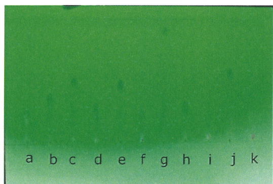
Figure 4. TLC analysis of the deprotonated rotaxane 1\text{H}_0\text{X}_0 in the presence of acids (eluent: \text{CH}_2\text{Cl}_2/\text{acetone}/\text{H}_2\text{O} , 3:16:1) under UV irradiation. Deprotonated rotaxane 1\text{H}_0\text{X}_0 in the presence of (a) \text{ClCH}_2\text{CO}_2\text{H} , (b) \text{Cl}_2\text{CH}_2\text{CO}_2\text{H} , (c) TFA, (d) \text{MsOH} , (e) \text{TsOH} , (f) (\text{CH}_2\text{SO}_3\text{H})_2 , (g) \text{HClO}_4 , (h) \text{HCl} , (i) \text{H}_2\text{SO}_4 , and (j) \text{HNO}_3 . (k) Deprotonated rotaxane 1\text{H}_0\text{X}_0 .
