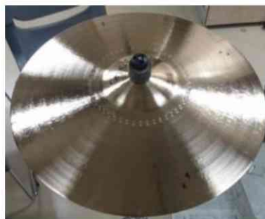
Fig. 5 Hammered cymbal with 50 dents on a 160 mm diameter circle.
