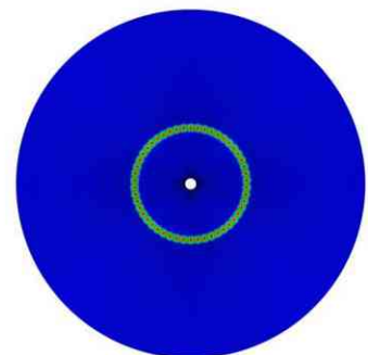
Fig. 6 Thermal loads corresponding to the hammered cymbal.
