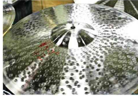
Fig. 3 Hammered cymbal having many dents on the surface.
