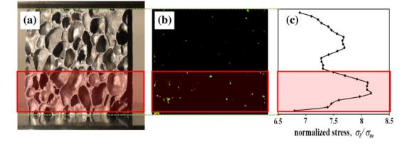
Fig. 7—Compressive behavior of ALPORAS specimen I (p = 88.9 pct) (previously shown in Figures 3 and 4): (a) initial pore structure, (b) stress distribution obtained by image-based FE analysis, and (c) mean stress distribution of planes obtained by image-based FE analysis.
