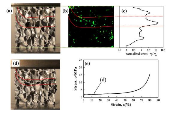
Fig. 8—Compressive behavior of ALPORAS specimen IV (p = 90.2 pct): (a) initial pore structure, (b) stress distribution obtained by imagebased FE analysis, (c) mean stress distribution of planes obtained by image-based FE analysis, (d) pore structure at compressive strain of  $\varepsilon = 12$  pct, and (e) stress–strain curve.
