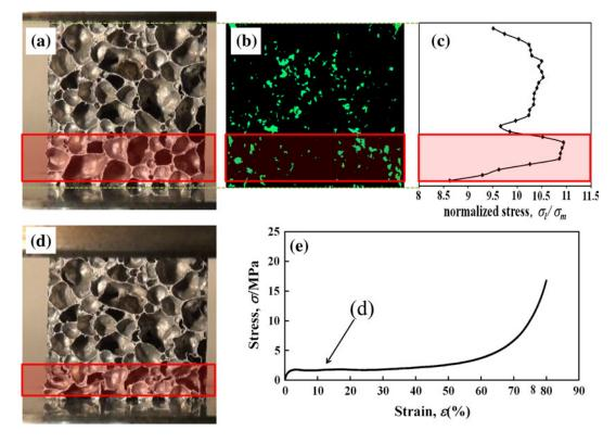
Fig. 6—Compressive behavior of ALPORAS specimen III (p = 89.8 pct): (a) initial pore structure, (b) stress distributions obtained by imagebased FE analysis, (c) mean stress distribution of planes obtained by image-based FE analysis, (d) pore structure at compressive strain of  $\varepsilon = 12$  pct, and (e) stress–strain curve.
