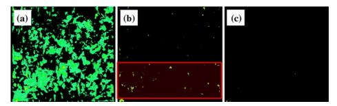
Fig. 4—Mises equivalent stress distributions for ALPORAS specimen I obtained by image-based FE analysis where the stress was greater than (a)  $2\sigma_{\rm m}$ , (b)  $3\sigma_{\rm m}$ , and (c)  $4\sigma_{\rm m}$ .
