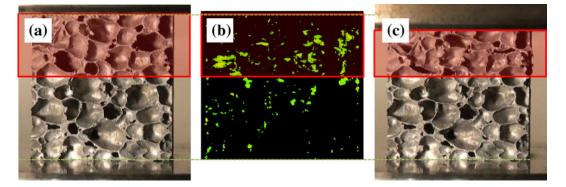
Fig. 5—Compressive behavior of ALPORAS specimen II (p = 88.8 pct): (a) initial pore structure, (b) stress distribution obtained by imagebased FE analysis, and (c) pore structure at compressive strain of  $\varepsilon = 12 \text{ pct}$ .
