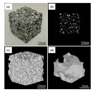
Fig. 1—(*a*) ALPORAS specimen used in compressive test. (*b*) Twodimensional cross-sectional X-ray CT image of ALPORAS specimen. (*c*) Voxel model of ALPORAS specimen. (*d*) Enlarged voxel model of ALPORAS specimen around pores.
