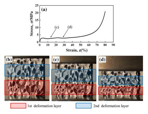
Fig. 3—Compressive behavior of ALPORAS specimen I (p = 88.9 pct): (a) stress–strain curve, (b) initial pore structure, (c) pore structure at compressive strain of  $\varepsilon = 12$  pct, and (d) pore structure at compressive strain of  $\varepsilon = 28$  pct.
