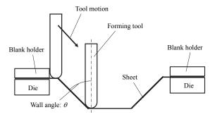
Fig. 3. Definition of wall angle.
