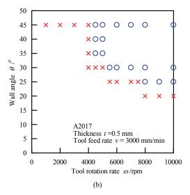
Fig. 4.(a) effect of tool rotation rate on formable wall angle. ( $\omega = 10000 \text{ rpm}$ ), (b) Effect of tool feed rate on formable wall angle. ( $\nu = 3000 \text{ mm/min}$ )
