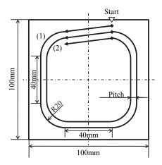
Fig. 2. Forming path and sequence.
