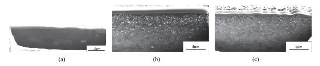
Fig. 5. Cross-sectional images of scanning ion microscope (v = 3000 mm/min,  $\omega = 10000$  rpm,  $\theta = 25$ °) (a) before forming, (b) parallel to tool travel direction and (c) perpendicular to tool travel direction.
