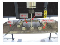
Fig. 1. Appearance of forming equipment.
