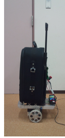
Fig. 4. Porter Robot based on Wheeled Inverted Pendulum Mobile System
