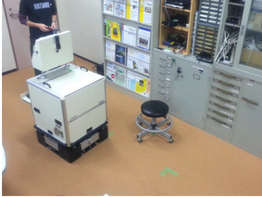
Fig. 7. Omni-directional vehicle embedded with 96 RFID readers on the bottom and experiment environment with RFID tag textile on the floor
