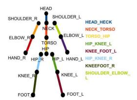
Fig. 1. Joint positions detected by Kinect
