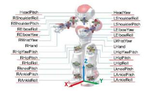
Fig. 2. Joints configuration of NAO (underlined joints are estimated by particle filter) and coordinate-system of NAO's CoM position. Draw and change from http://doc.aldebaran.com/2-1/family/nao\_dcm/ actuator\_sensor\_names.html
