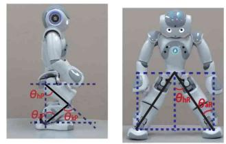
(a) Joints angle of pitch in lowerbody (b) Joints angle of roll in lower-body
