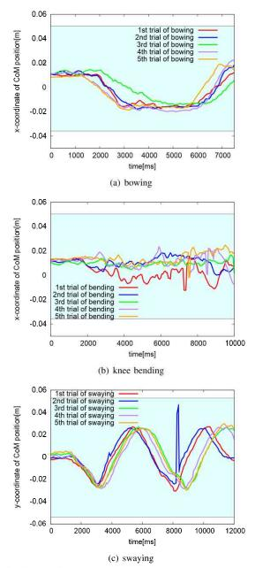
Fig. 13. CoM position of the NAO during imitation: In case (a) the bowing motion and (b) the knee bending motion, the movements of CoM in back and forth (x-axis) direction are shown. In case of (c) the swaying motion, the movements of CoM in side(y-axis) directio are shown.
