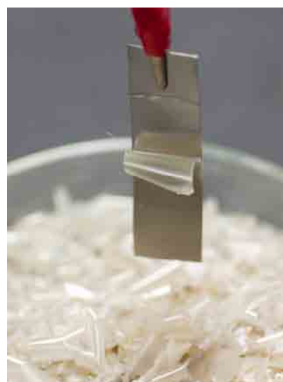
Fig.1 Photograph showing TiO 2 nanotube array film peeling off from Ti plate.
