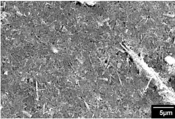
Fig.6 SEM image of hybrid TiO 2 nanoparticle / nanotube film.
