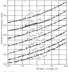
Fig.6 Relation between atmospheric pressure and bridge voltage
