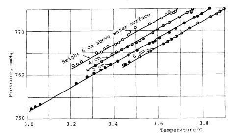
Fig.2 Variation of indicating temperature due to deviation of positions of the thermometer valve above the water surface
