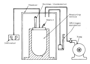
Fig.5 Experimental apparatus for test of the measuring device
