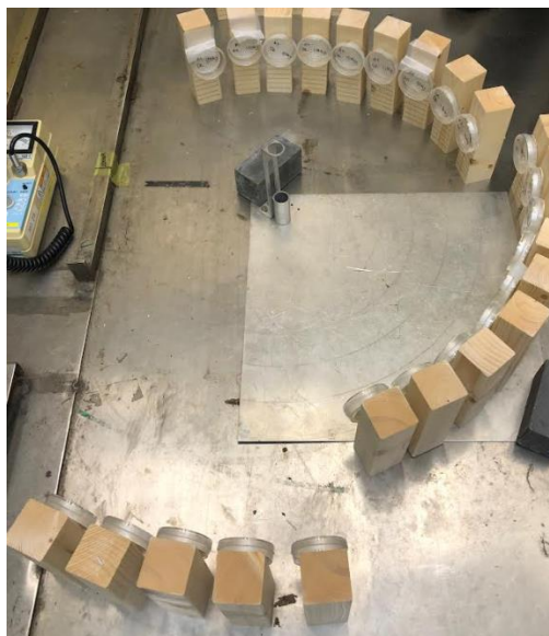
Figure 6.4 The arrangement of samples for gamma irradiation
