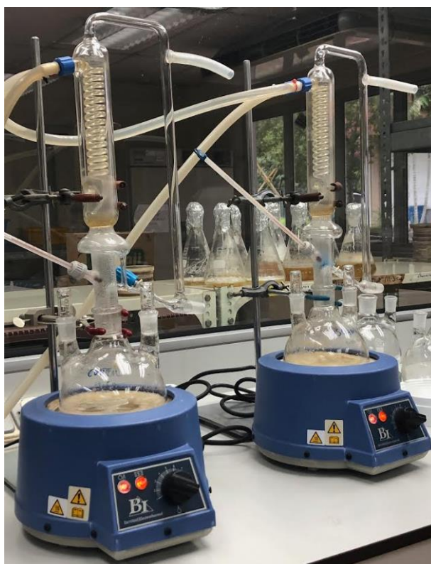
Figure 5.1 Setup of reflux extractor for water extraction
