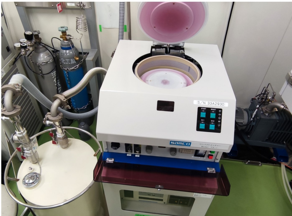
Figure 18. Compact Etcher setup [SAMCO FA-1].
