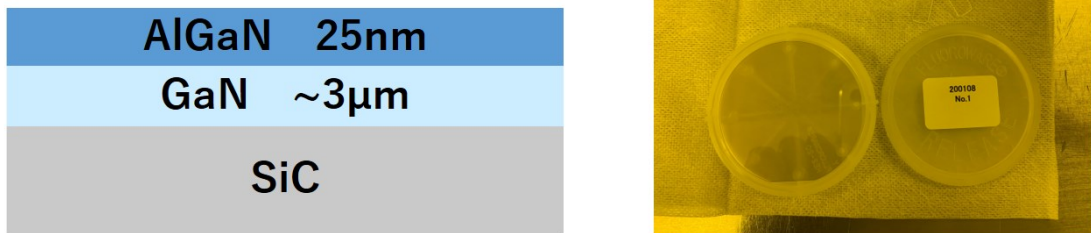
Figure 1. Structure of the wafer (left) and its packaging (right)
