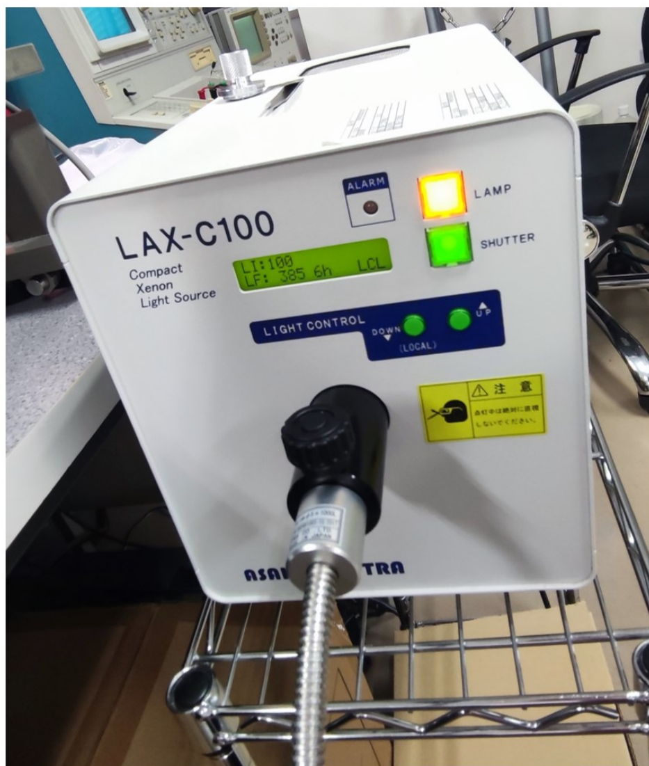
Figure 22. Monochromatic light source [LAX-C100].
