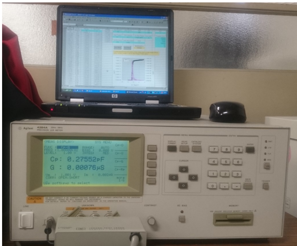
Figure 21. Capacitance-Voltage measurement system [Agilent 4284A].
