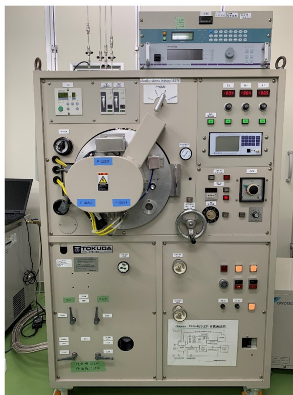
Figure 16. RF plasma sputtering setup [TOKUDA CFS-4ES].
