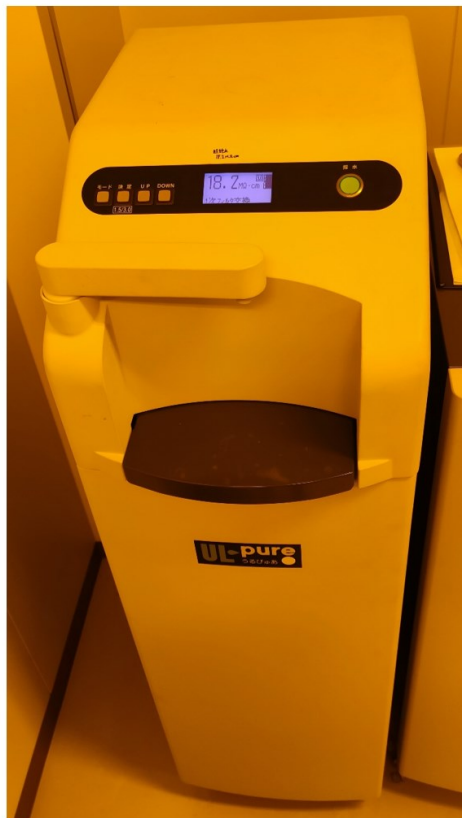
Figure 19. Deionized water plant [UL-pure with storage tank]
