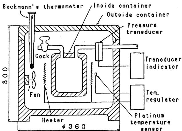
Fig.1 Structure of temperature-controlled device
