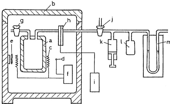
Fig.11 Measuring device of barometric difference
