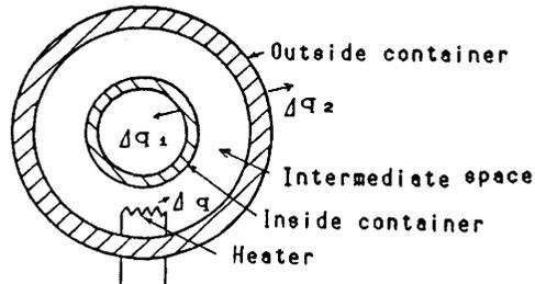
Fig.3 Physical model of temperature-controlled device
