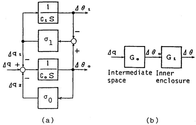
Fig.4 Block diagram of heat transference
