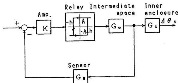
Fig.5 Block diagram of temperature-controlled system
