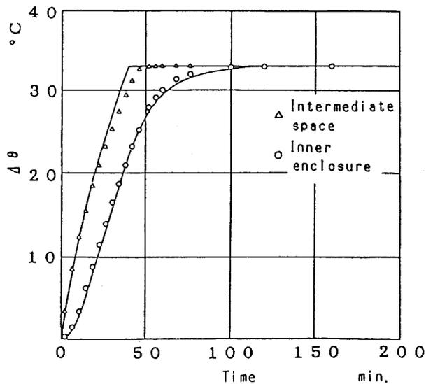
Fig.7 Transient response of temperature-controlled device
