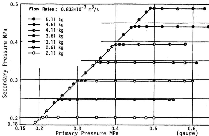
Fig.8 Pressure-adjustment characteristics
