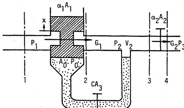
Fig.2 Sketch of plunger-type control valve
