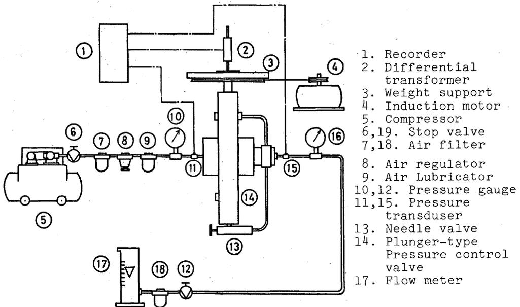
Fig.5 Experimental apparatus
