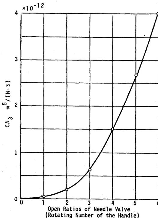
From these results, values of  $CA_3$  were obtained and then the relationship between rotating number of the needle valve and  $CA_3$  was shown in Fig.6. Figure 6 illustrates that the value  $CA_3$  can be obtained by the rotating number of the needle valve.
