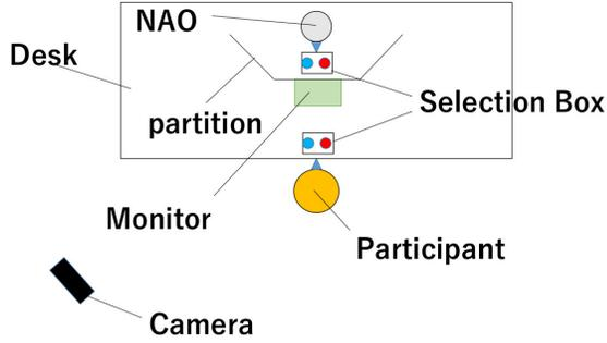
Fig. 4. Arrangement of the experimental equipment
