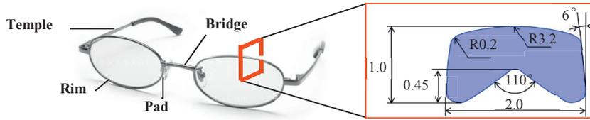
Fig. 1. Names of glasses frame parts and sectional shape of wire.
