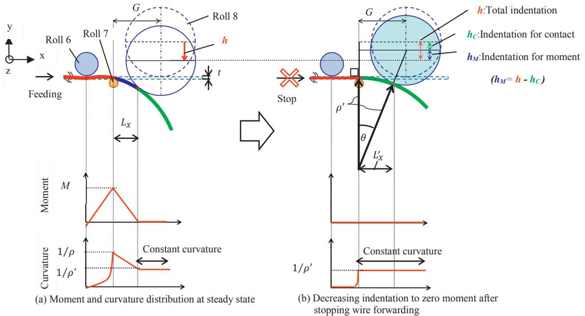
Fig. 4. Illustration of steady bending process.
