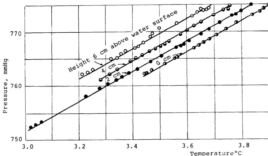
Fig.2 Variation of indicating temperature due to deviation of positions of the thermometer valve above the water surface
