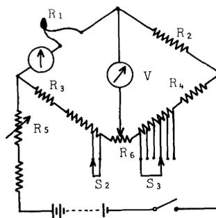
Fig.4 Temperature measuring circuit
